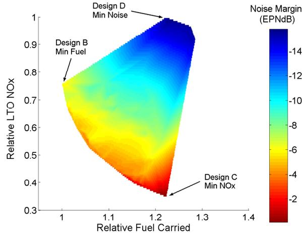
Figure 12. Pareto surface of LTO NO<sub>x</sub> vs. Fuel Carried vs. Cumulative Noise. Only rank 1 designs are shown.
