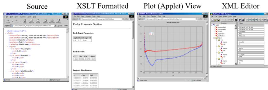
Figure 4. Data is represented in CAFFE in an internal data structure and with a persistent XML database, easily presented to users in many forms.
