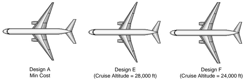
**Figure 13. Top view of aircraft optimized for cruise at altitudes of 28,000ft (Design E) and 24,000 ft (Design F) with minimum cost Design A.**
