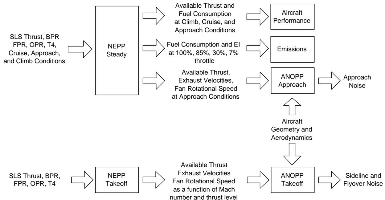
Figure 9. ANOPP and NEPP integration in the framework.
