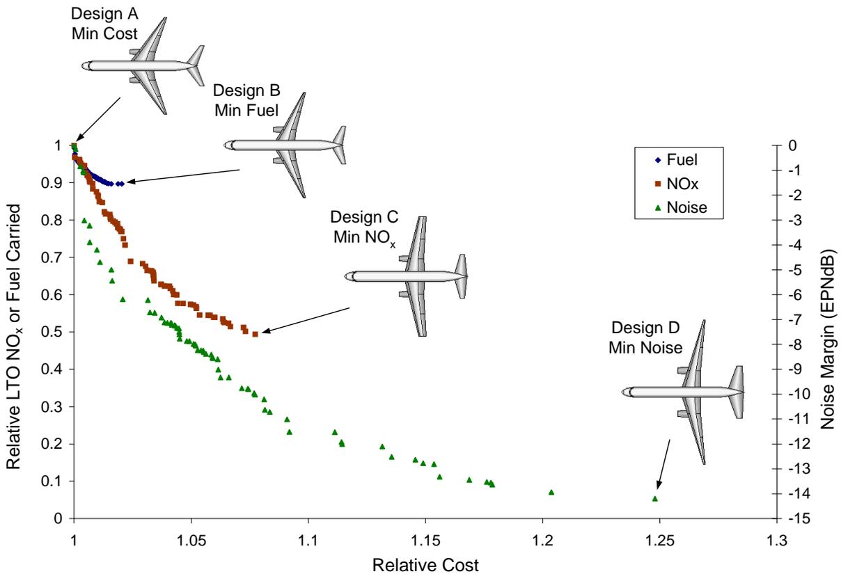
Figure 10. Pareto fronts of fuel carried, LTO NO<sub>x</sub>, and cumulative certification noise vs. operating cost. Only rank 1 designs are shown. Average rank for all fronts is under 4.
