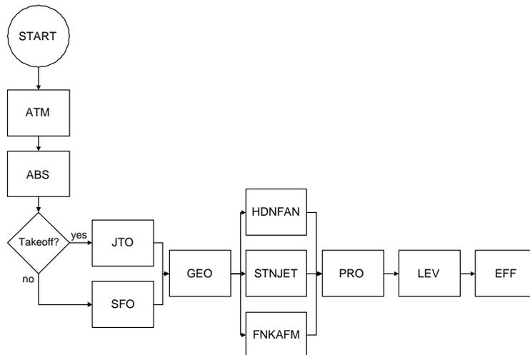
Figure 8. Flow chart of ANOPP program modules.
