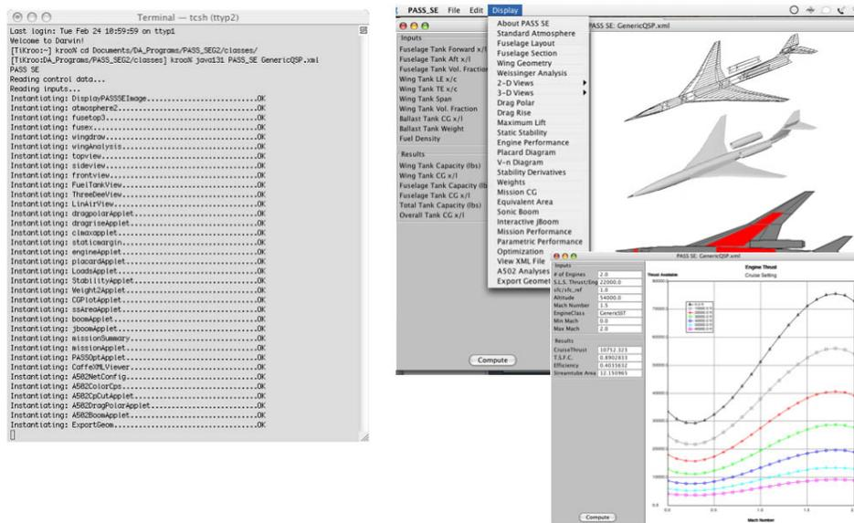
Figure 7. Interfaces may be customized – from simple command-line interaction to custom user interfaces, CAFFE defines an API, not just for analyses, but for user display and interaction.
