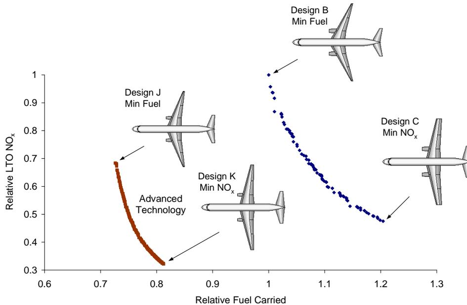
Figure 14. The benefits of increased laminar flow, reduced induced drag, and lower structural weight are illustrated on the fuel-cost Pareto front.
