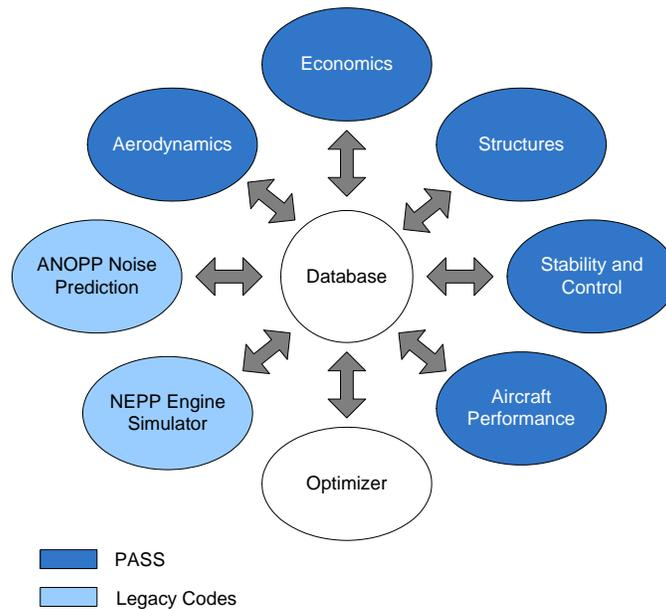
**Figure 2. Elements of the Aircraft Conceptual Design Framework**
