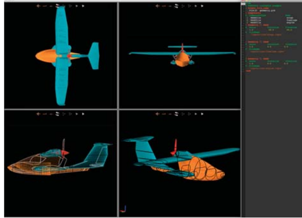
Figure 7. Extended version of the original RAGE interface developed to display a provided 3-view as an underlying canvas.
